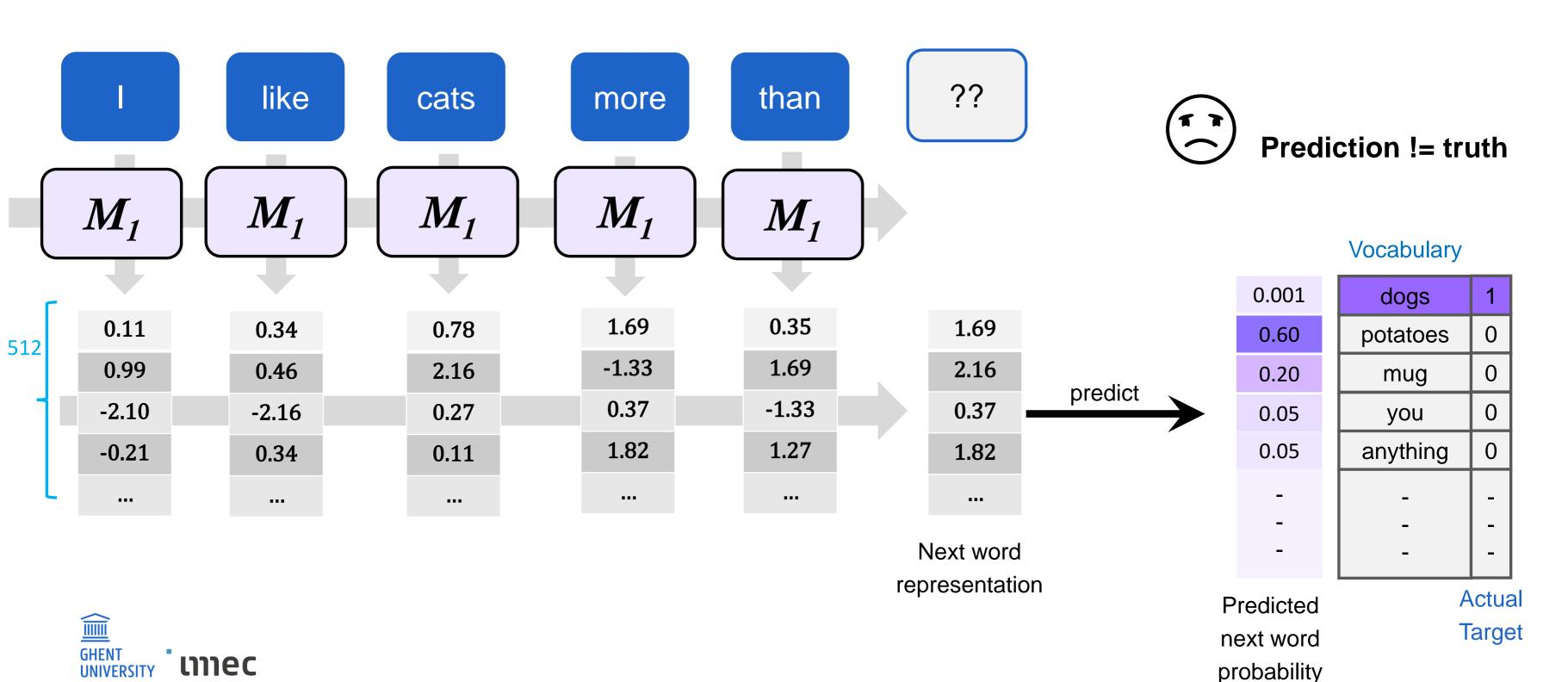
Calculate the error (loss) between the prediction and the actual target
